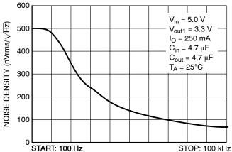
Figure 11. Noise Density vs. Frequency
