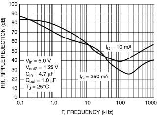
Figure 10. Ripple Rejection vs. Frequency for Vout2
