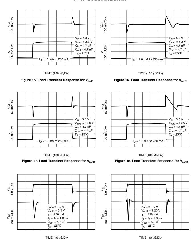
Figure 19. Line Transient Response for Vout1
