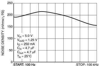
Figure 14. Noise Density vs. Frequency
