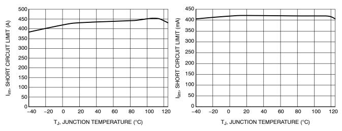
Figure 7. Short Circuit Current Limit vs. Temperature for  $V_{out1}$
