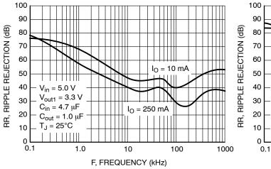
Figure 9. Ripple Rejection vs. Frequency for  $V_{out1}$
