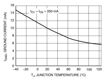
Figure 6. Ground Current vs. Temperature
