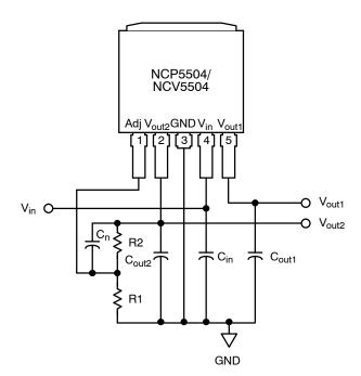
Figure 1. Application Schematic, Fixed Output Version.  $V_{out1}$  = 3.3 V,  $V_{out2}$  = 1.25 V
