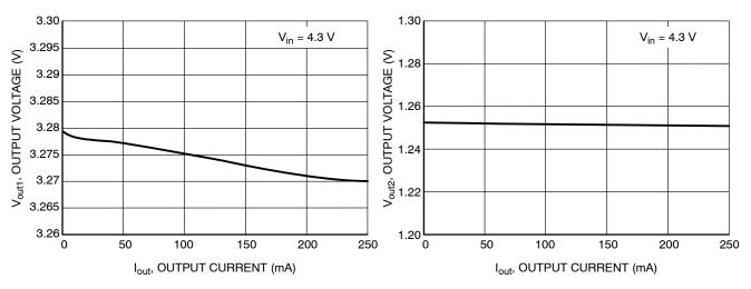
Figure 3. Output Voltage vs. Output Load Current for V<sub>out1</sub>
